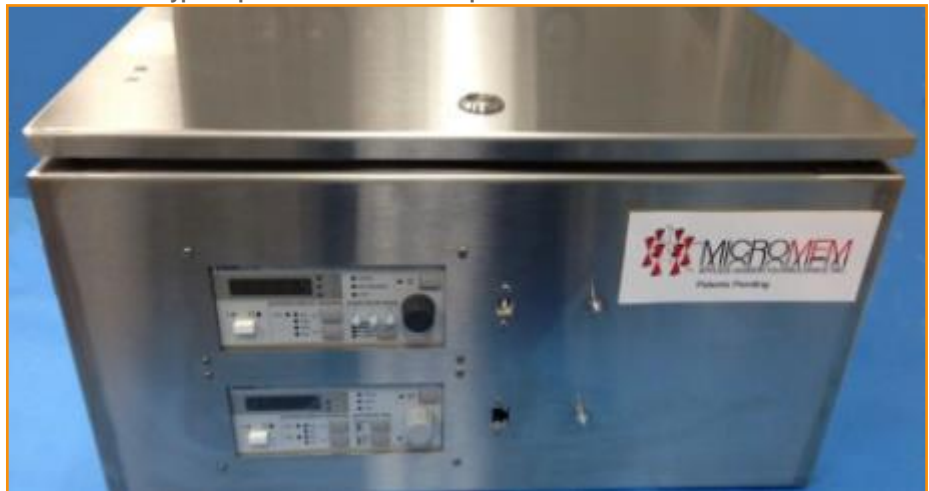
Exhibit 4: Prototype of product to detect nanoparticles in oil
